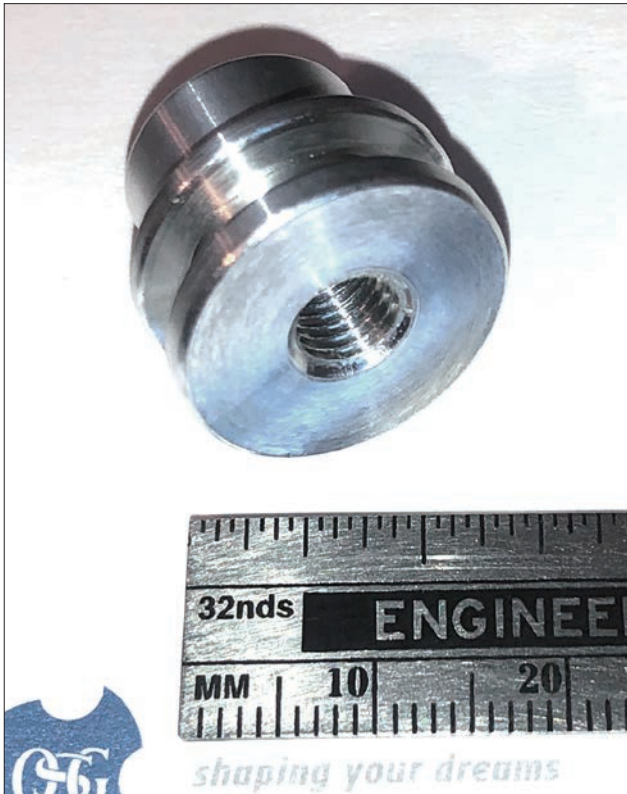
Flickinger Industries produces aluminum air cylinder pistons in sizes ranging from 1/2" diameter up to 3" diameter and in lot sizes of typically 2,000 to 5,000 pieces – totaling over 1 million pistons per year. The parts are made from T356 aluminum bar stock and each piston has a threaded center hole.
