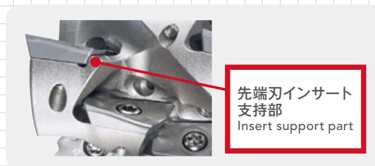
2段目以降：切れ味重視配列 2nd and subsequent steps: for high sharpness
