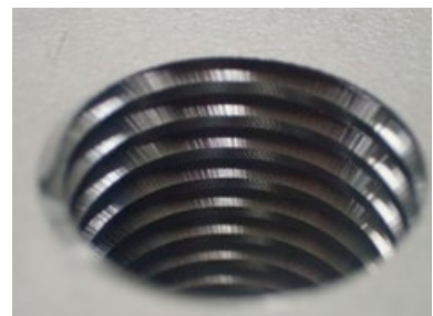
従来品 (2パス) Conventional Thread Mill 2-pass
