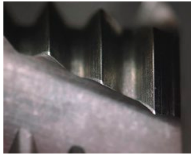
1本目 8,800穴加工後 No.1 (after cutting 8,800 threads)
