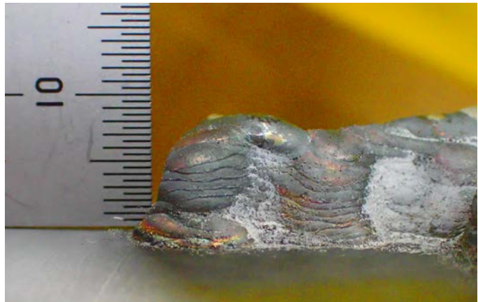
Figure 3. Photograph of deposit by the DED method in SKD11 (60 HRC)
