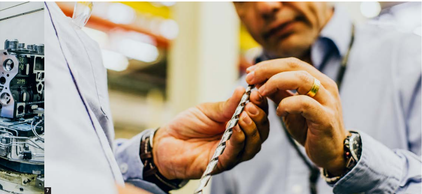
7. MWM Process Engineer Tarcisio Bottaccini inspects the 8 mm diameter ADO 30xD next generation high performance carbide drill.
