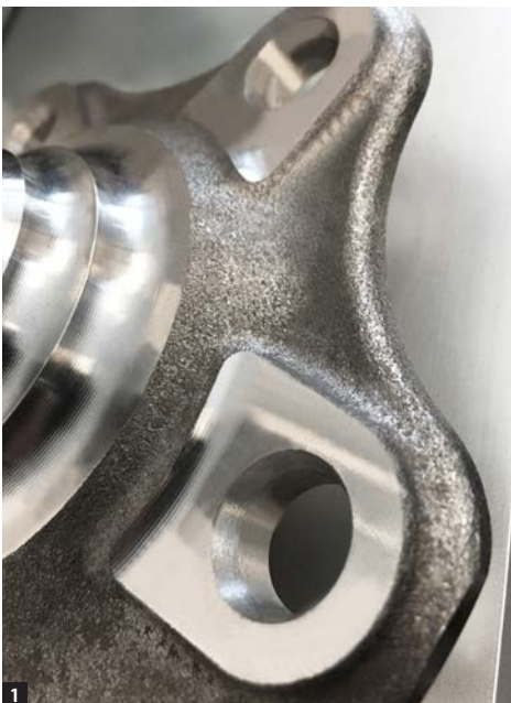
1. Each of NTA's wheel hub bearing requires the drilling of five holes in grade S53C carbon steel. NTA produces approximately 840,000 parts per year, accounting for 4,200,000 drilled holes annually.
