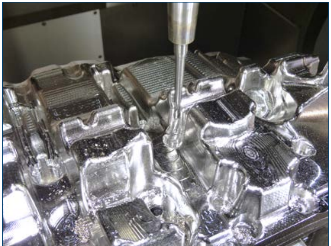
Right: Meissner often works with components with tight pockets, narrow webs and high contours, which can limit the swiveling movements of the machining center, resulting in a reduction of speeds and feeds.
