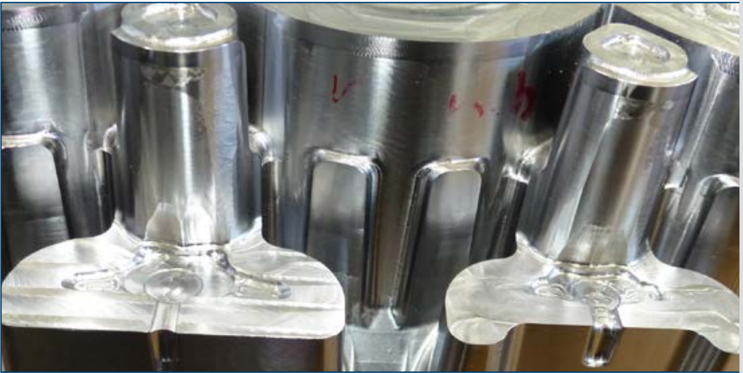
With the implementation of OSG's end mill tooling, it has been proven that even 3-axis machining can be significantly more efficient than 5-axis milling when processing water jacket core tools with deep and narrow cavities.
