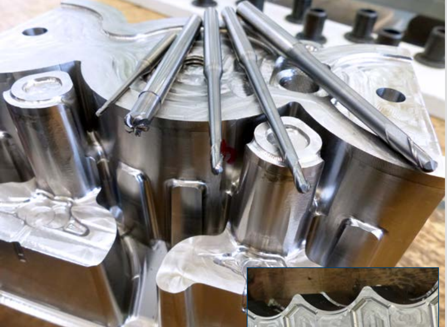
Above: Meissner's parts require a tolerance of 0.03mm, which OSG's end mills are able to achieve the required precision consistently.
