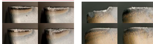
PSTW (4m加工時点) After machining 4m
