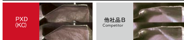
[FCD600] 1,600穴加工時の摩耗比較 Wear comparison after 1,600 holes of drilling
