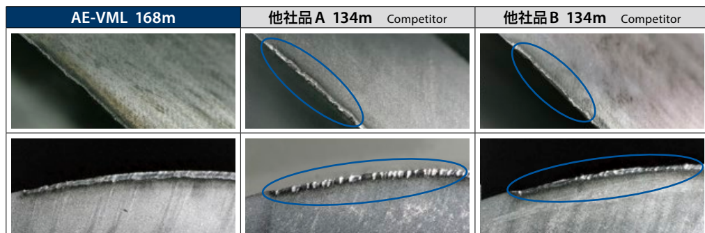
外周刃の損傷状態 Wear comparison of the peripheral cutting edge
