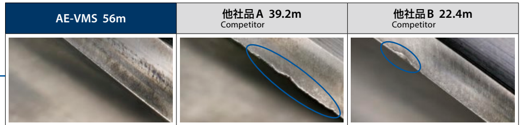
外周刃の損傷状態 Wear comparison of the peripheral cutting edge
