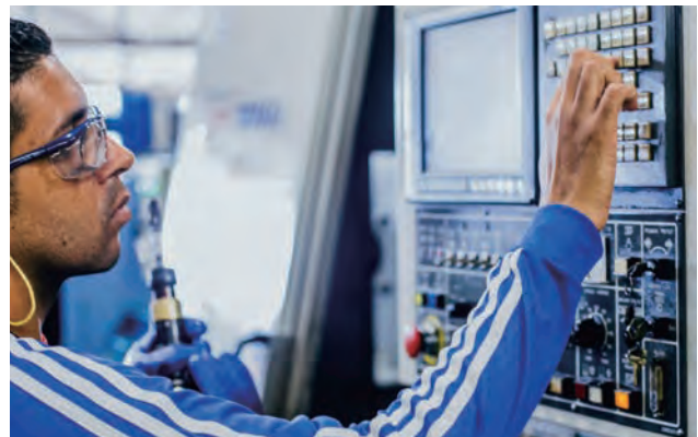
ZF's machine operator prepares for the machining of automotive pipes using a Doosan MV3016LS vertical machining center.
