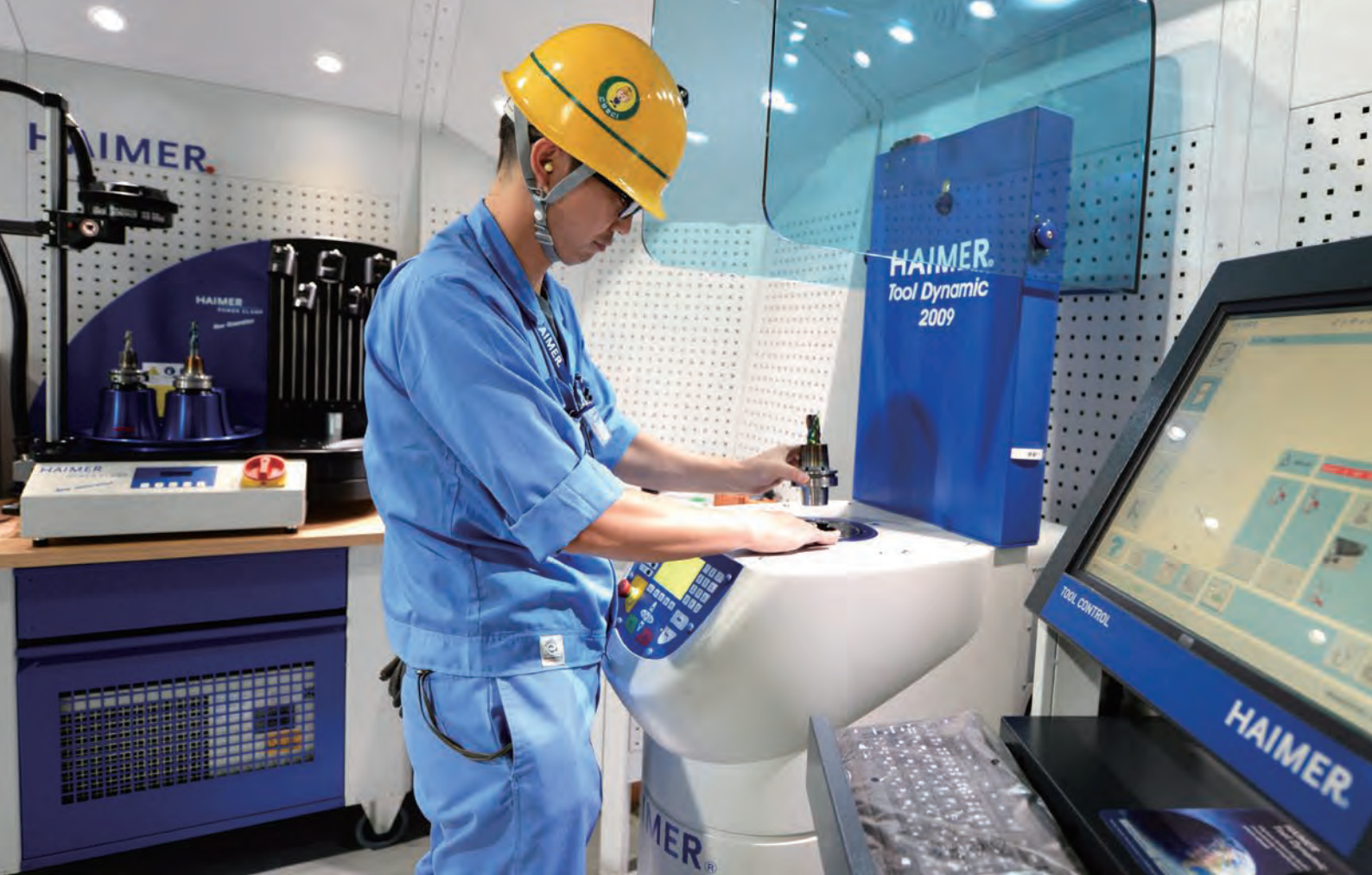
Takanori Terasako, MHI technician and a member of the 777X project, uses the HAIMER Tool Dynamic balancing machine at the Eba Factory in Hiroshima.
