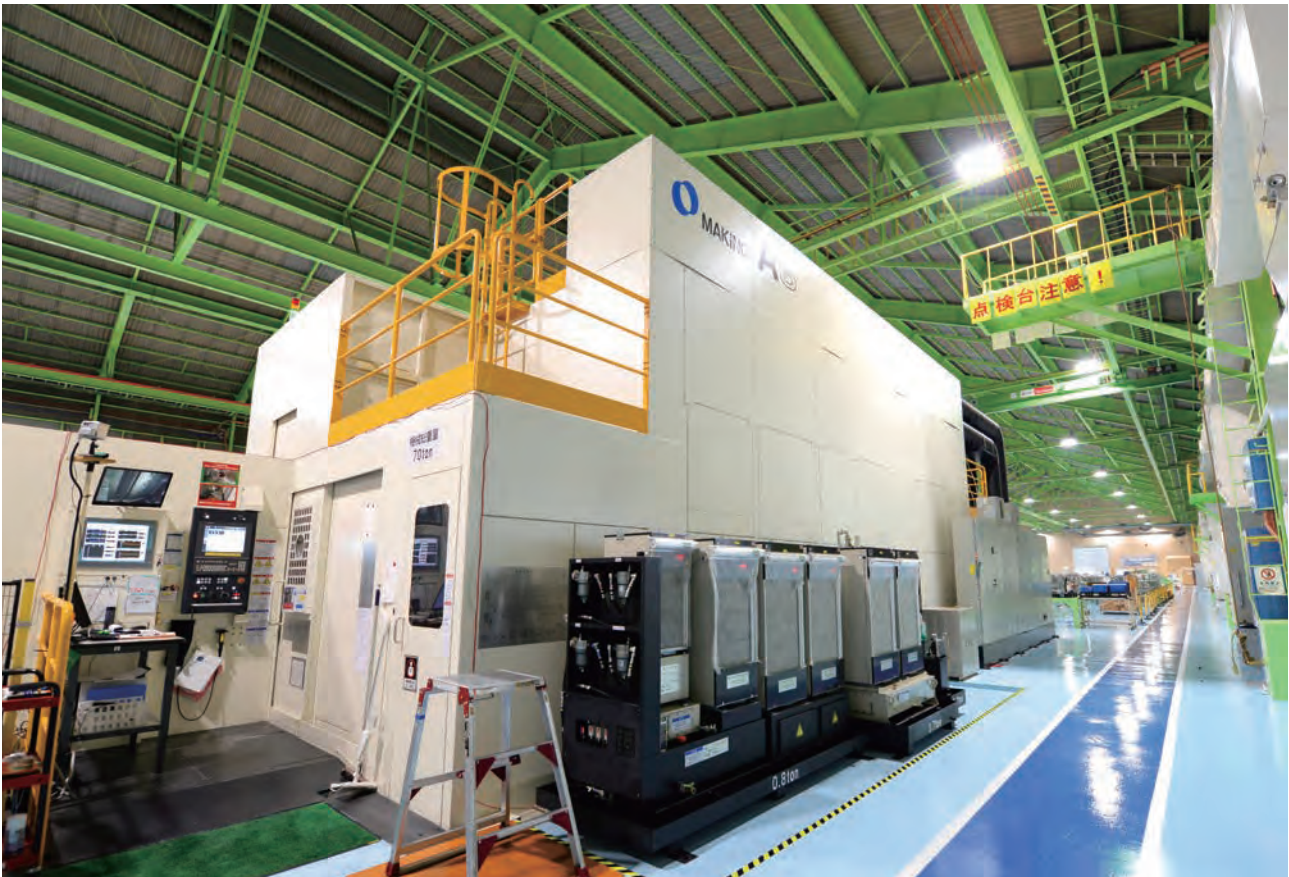
With the launch of the Boeing passenger aircraft 777X project, MHI decided to introduce a 120 kW high-speed and high power 5-axis horizontal machining center, the Makino A6, with a maximum spindle speed of 33,000 min -1 to improve productivity substantially.
