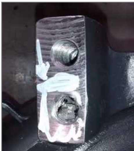
Tap breakage was a headache for Scania before switching to the XPF forming tap.
