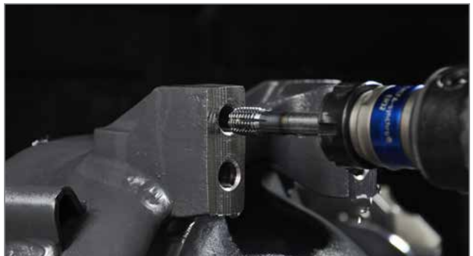
The XPF is OSG's high performance form tap that produces no chips and is optimized for machining materials up to 35 HRC.
