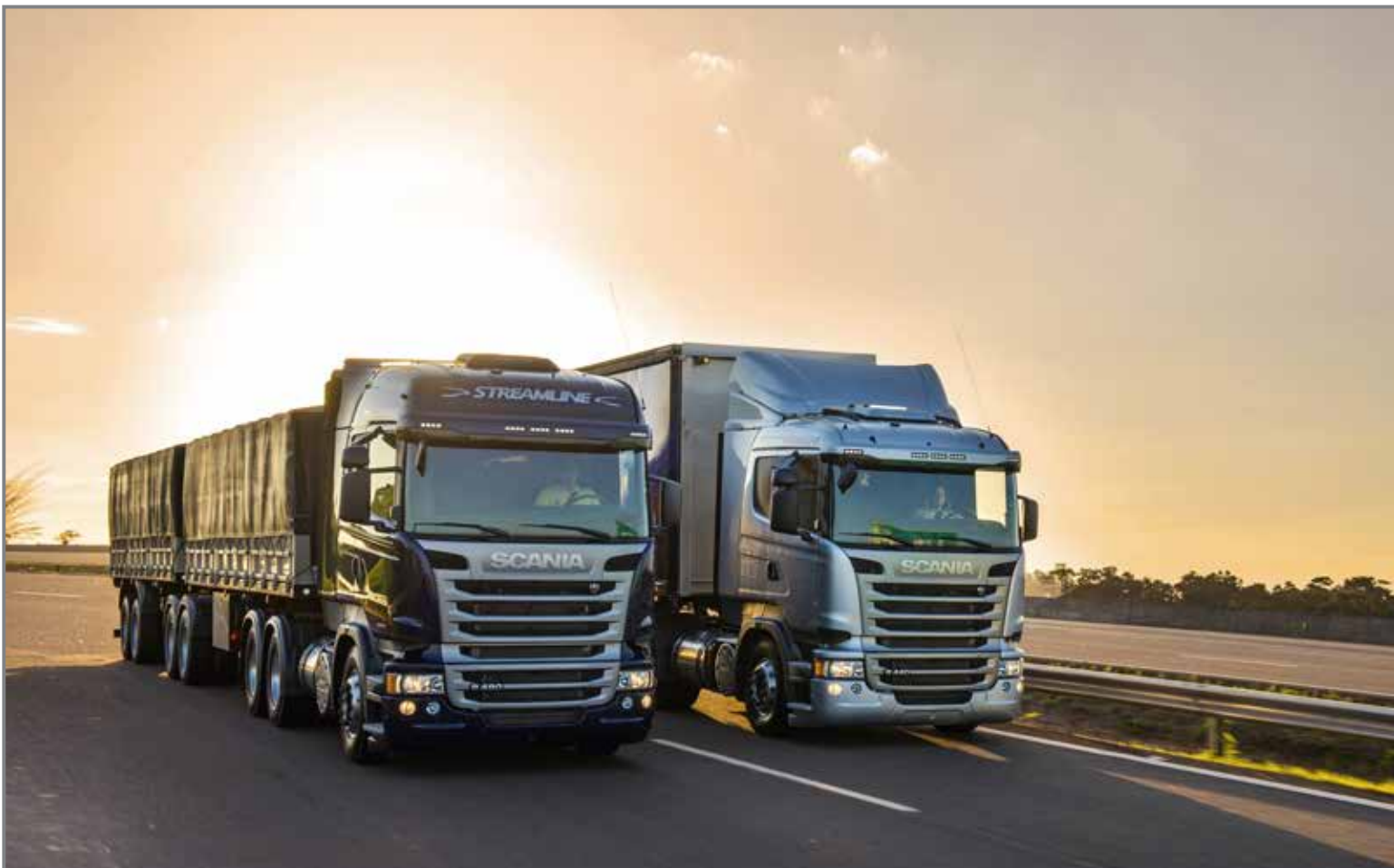
Scania R 480 6x4 Streamline, Highline cab with B-double combination and Scania R 440 6x4 Streamline with general cargo. Photo courtesy: Scania.
