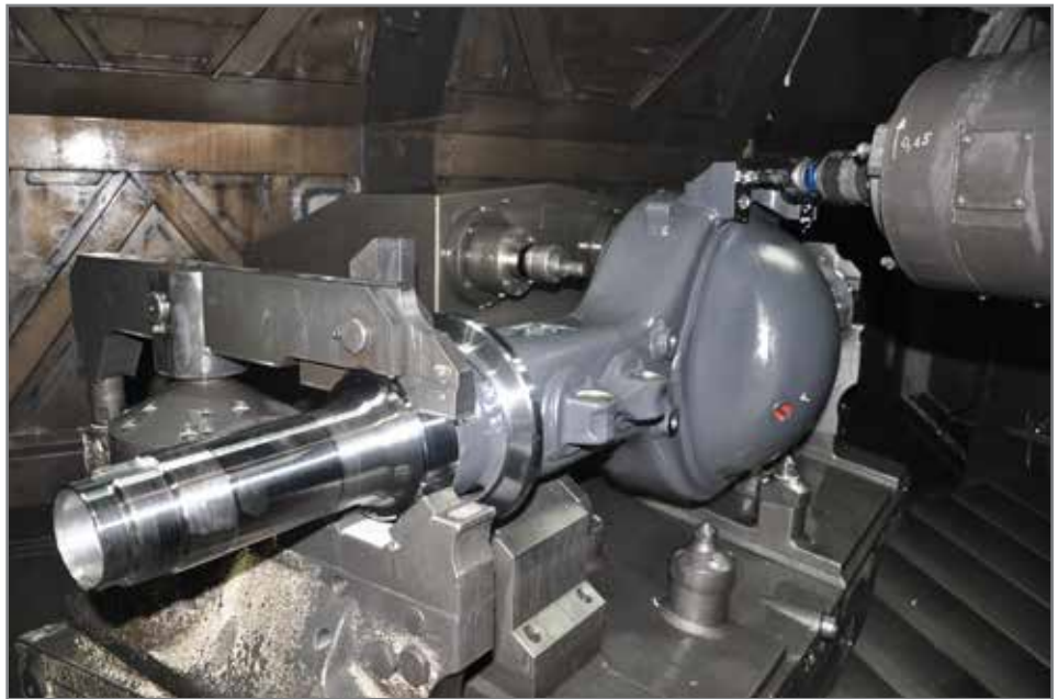
The XPF form tap is used for machining the threads of the differential housing.
