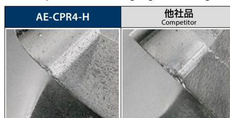
1,512m 加工後の刃先の損傷状態 Wear comparison of the cutting edge after milling 1,512 m
