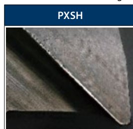
38.5m 加工後の刃先の損傷状態 Wear condition of the cutting edge after milling 38.5m
