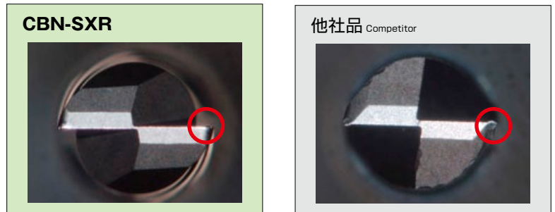
50m加工後の刃先状態 Cutting edge condition after machining 50m.
