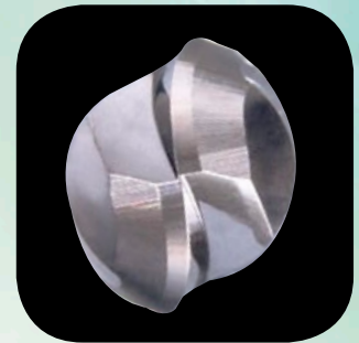
再研磨後 After regrinding
